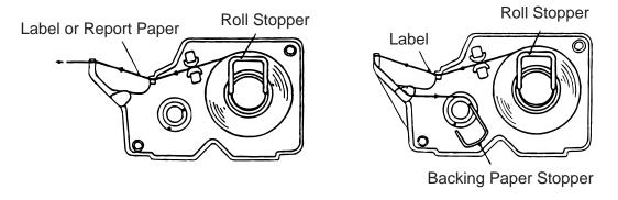
9. Assemble the label cassette to the scale and remove slack of the media. Push down the print head, and close the right cover.
